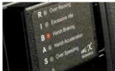
MIX Telematics's FMCommunicator Unit, placed in the first ethanol-powered bus in South Africa, is used worldwide and can monitor fuel consumption to calculate CO 2 emissions
