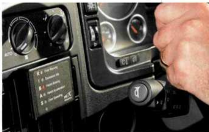
MIX Telematics's FMCommunicator Unit, placed in the first ethanol-powered bus in South Africa, is used worldwide and can monitor fuel consumption to calculate CO 2 emissions
